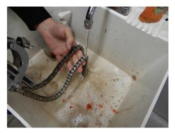
**Two**: Dry completely by laying out, with compressed air or with dry cloth.
