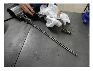
**Three**: Lubricate all moving parts with light oil removing all excess oil before stowage.
